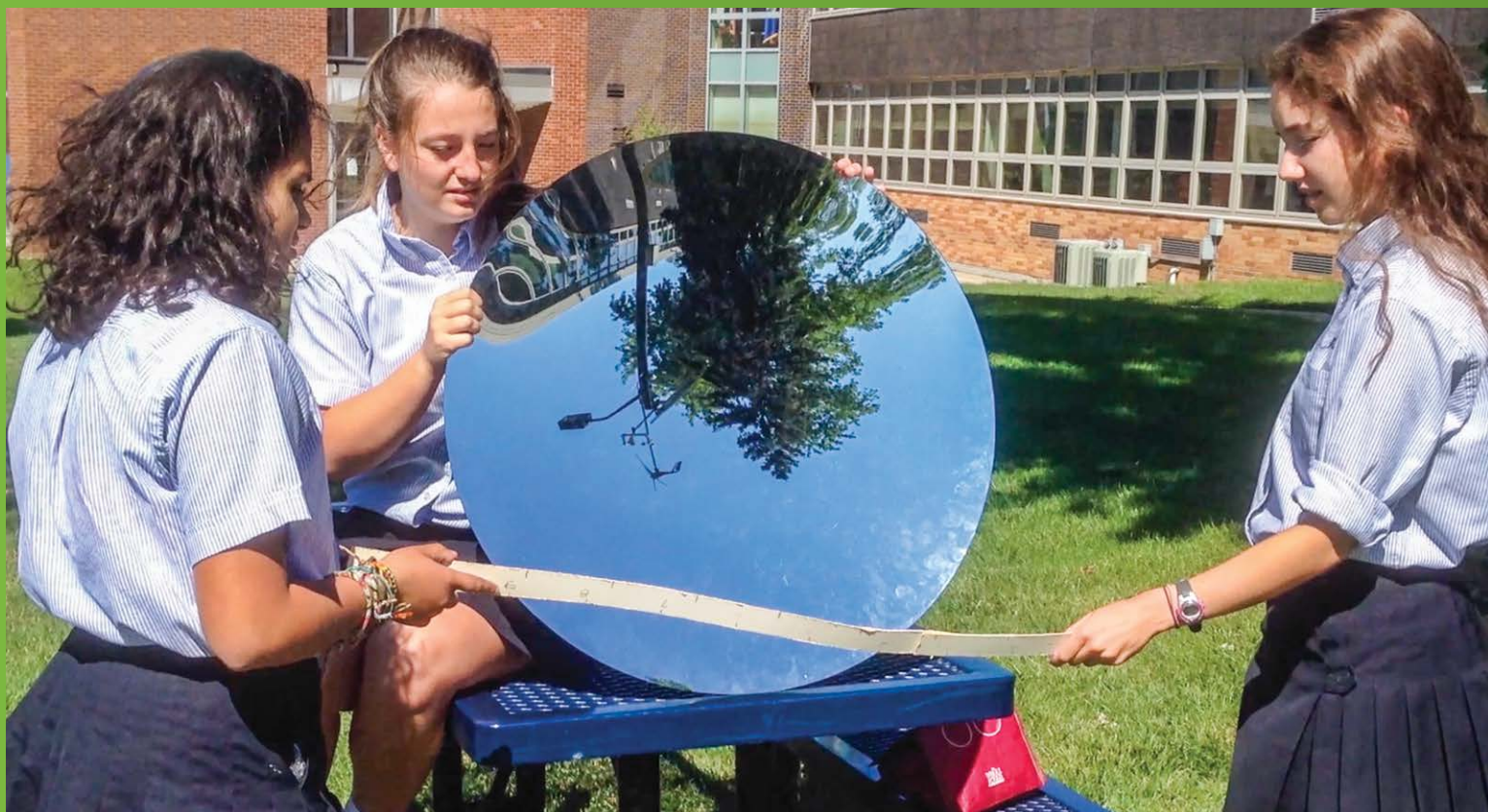
Figure 1. Testing a parabolic reflector to enhance the efficiency of a novel apparatus to produce biochar.
